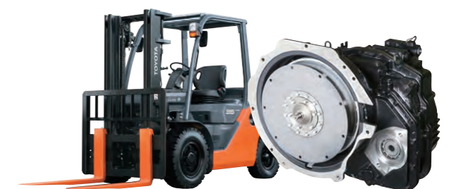
Torque converter type transmission for forklifts
